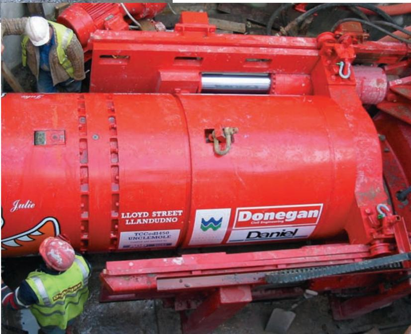
1,200mm dia. slurry microtunnelling system used to install
