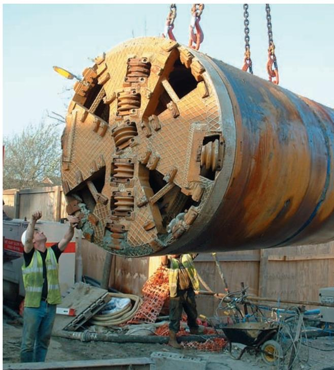
Condition of 1800 EPBM on completion of second drive (courtesy Southern Water).
