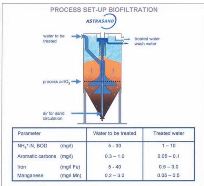
Process set-up Biofiltration (courtesy Paques)
