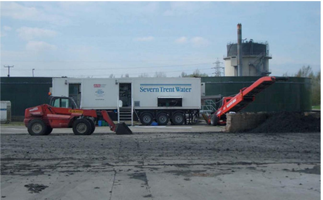
Mobile containerised dewatering plant
