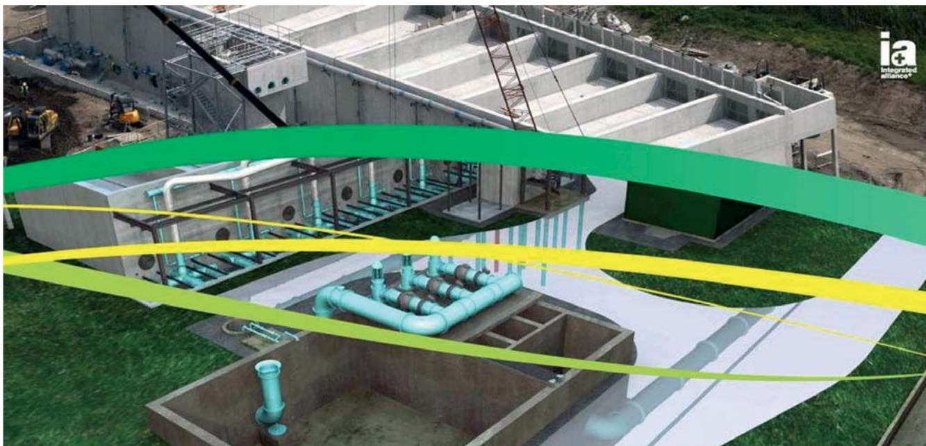
3D image of BAFF - Pumping Station; Distribution Chamber and BAFF Cells
